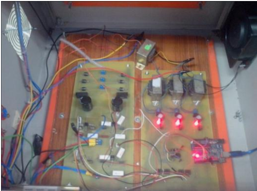
Figure 7a Hardware circuitry of prototype Hybrid NPC Inverter
