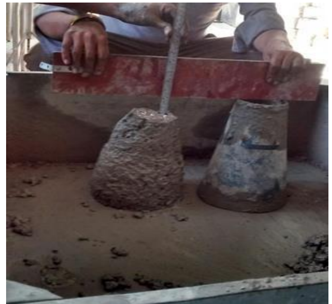
Fig.1 Workability Measured by Slump Test
