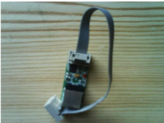
Fig 3 show the USB to serial converter to PC
