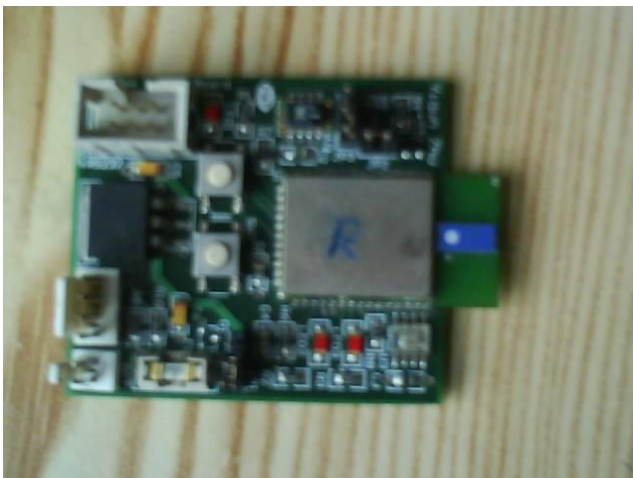
Fig 2 A zigbee sensor board Router Device (Label R)
