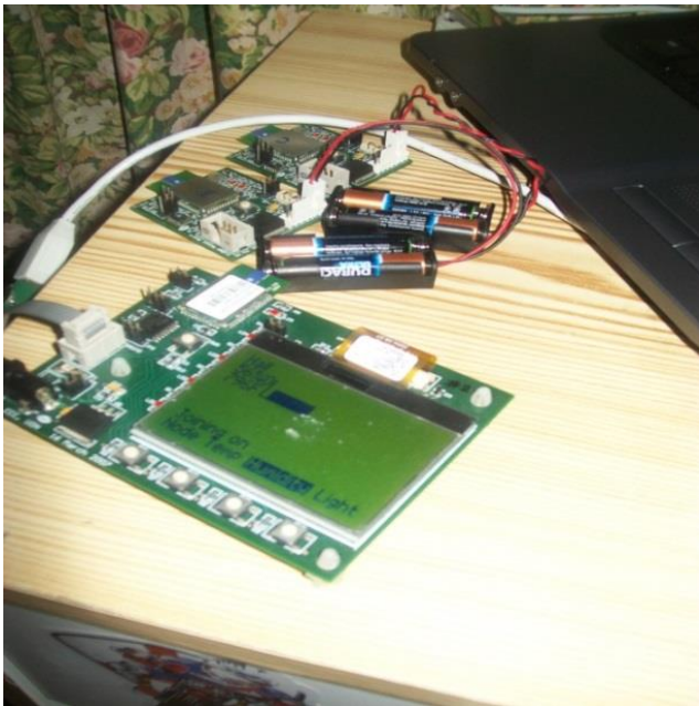
Fig 9 Controller Board showing the Humidity reading
