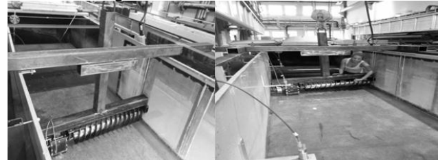
Fig. 12. Views of the new 3-bladed horizontal axis Archimedean screw turbine inside a long channel
