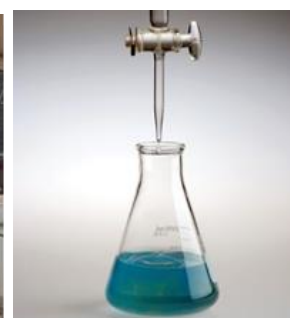
Figure 5b. Complete Titration (Lardbucket, 2013)
