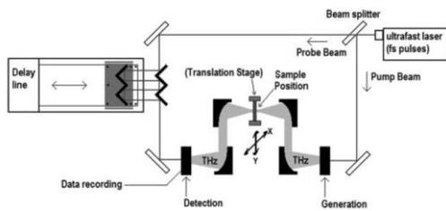
Figure (2): Configuration of a THz-TDS apparatus for transmission measurements [7].
