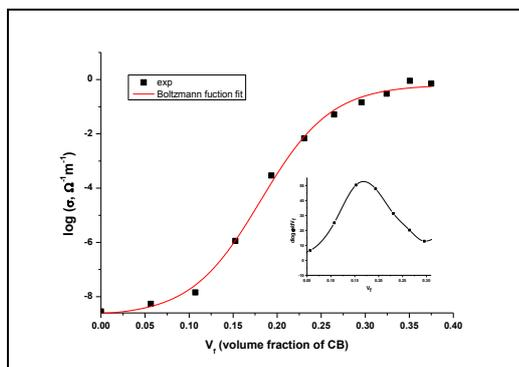
Figure (3): The variation of DC conductivity of CB loaded NBR composites (0-100 phr).
