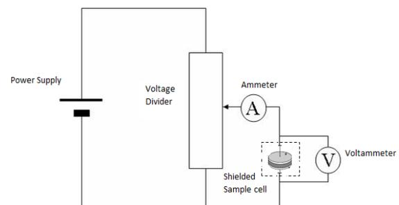
Figure (1): Schematic diagram of the circuit used for DC conductivity and I-V measurements.
