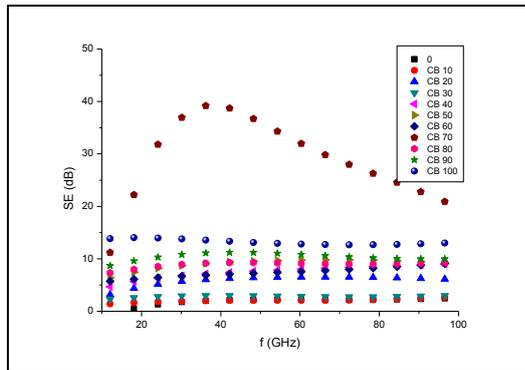
Figure (7): Shielding effectiveness for CB loaded NBR composites in the frequency range 10-100 GHz.
