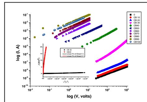
Figure (4): The I-V characteristic curves for the CB loaded NBR samples at 300K plotted on a log-log scale. The inset shows the relation of  $J$  versus  $V^2$  for CB30 and CB40 samples.
