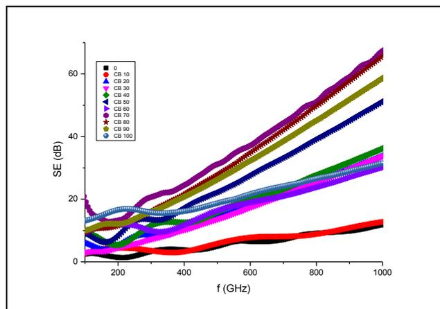
Figure (8): Shielding effectiveness for CB loaded NBR composites in the frequency range 100-1000 GHz.
