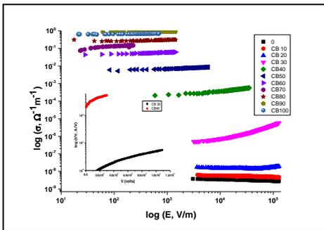
Figure (5): Variation of DC conductivity with electric field plotted on a log-log scale for CB loaded NBR samples (0-100 phr) at 300K. The inset shows the relation of  $\log I/V$  versus  $V$  for CB30 and CB40 samples.
