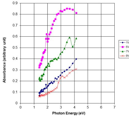
Figure 2 Spectral absorbance of ZnS films deposited at different applied voltage.
