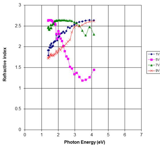
Figure 4 Plot of refractive index versus photon energy for the films deposited at 1V, 5V, 7V and 9V.
