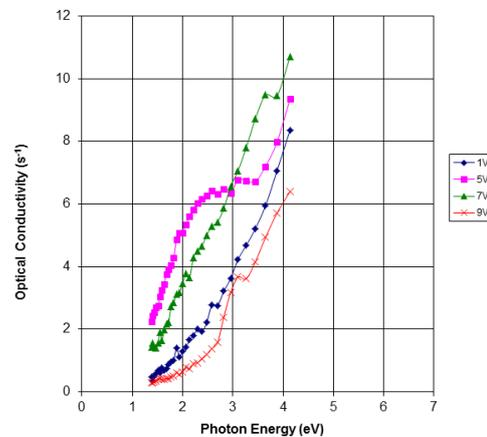
Figure 6 Plot of optical conductivity versus photon energy for the films deposited at 1V, 5V, 7V and 9V.
