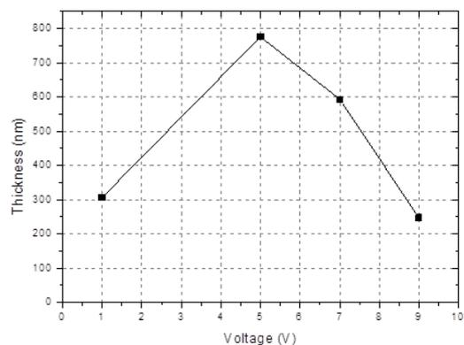
Figure 1 Plot of the thickness of the deposited films versus applied voltage.
