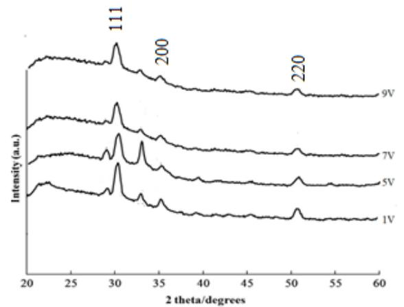
Figure 10 X-ray diffraction patterns of ZnS thin film deposited on conducting glass (ITO) substrate at various applied voltage.
