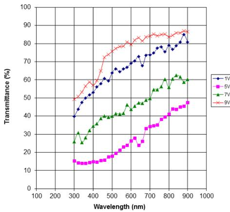
Figure 3 Spectral transmittance of ZnS films deposited at different applied voltage.
