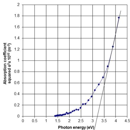
Figure 9 Plot of  $\alpha^2$  versus photon energy of deposited ZnS film.
