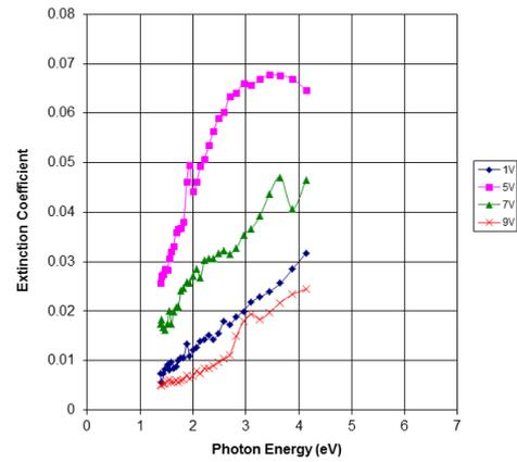
Figure 5 Plot of extinction coefficient versus photon energy for the films deposited at 1V, 5V, 7V and 9V.
