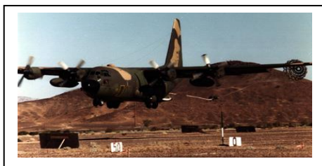
a. Drogue parachute is ejected into the airstream
