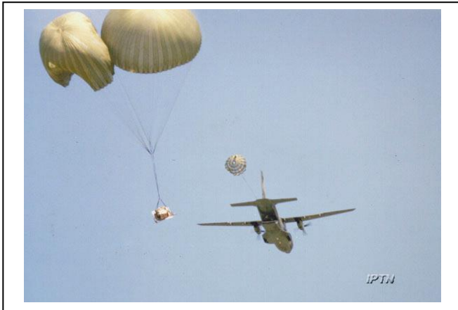
Fig. 8. CN-235 during LAPES
