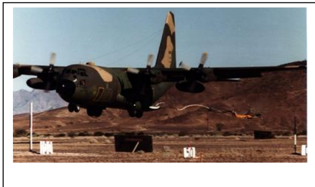
b. Cluster of parachutes extracted from deployment bag
