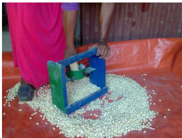
Fig. 2. Shelling activity using adjustable hand maize sheller
