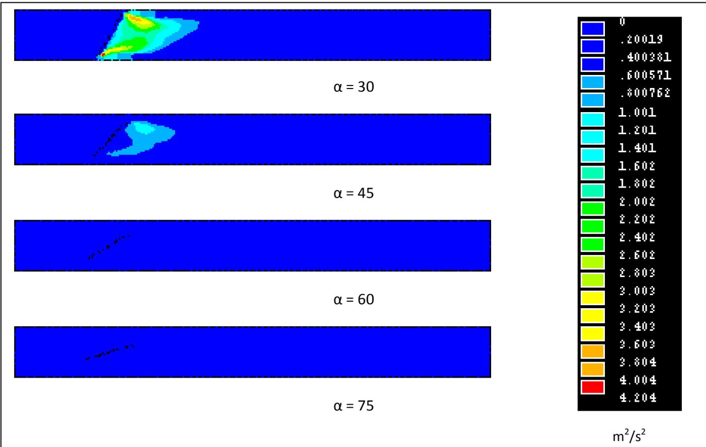
Fig.10: Change of turbulent kinetic energy with opening angles for 1 m/s inlet velocity
