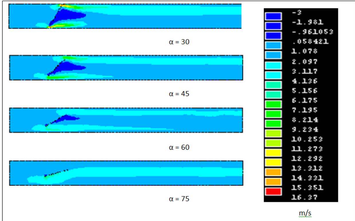
Fig.3: Change of velocity profile with opening angles for 2 m/s inlet velocity
