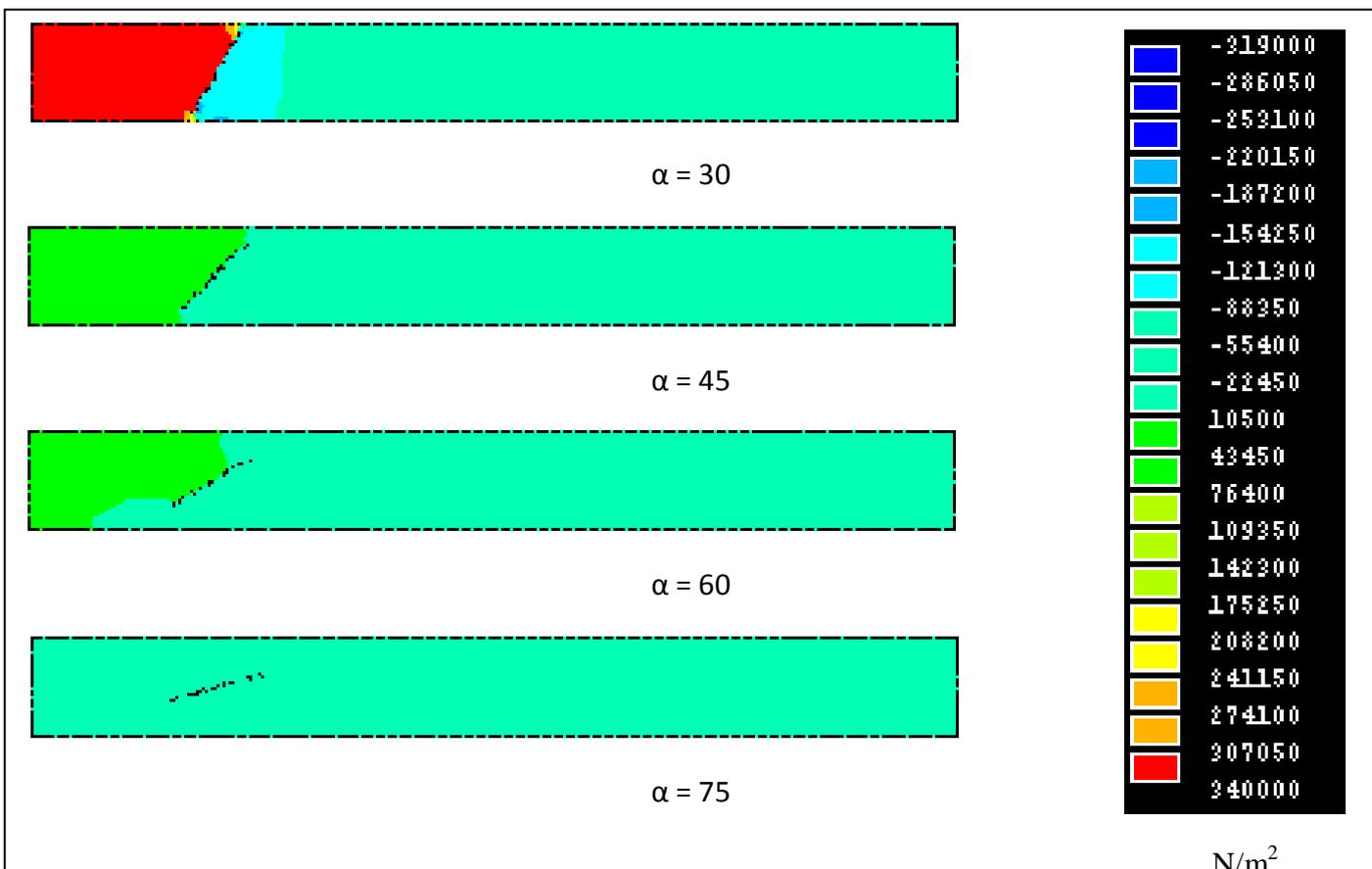
**Fig.9:** Change of pressure distribution with opening angles for 4 m/s inlet velocity
