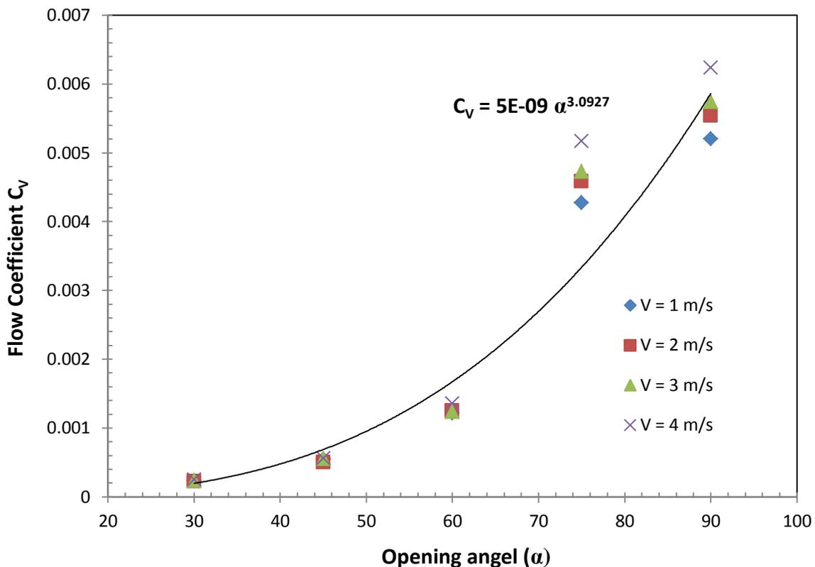
**Fig.14:** Variation of loss coefficient with opening angle at different flow velocities
