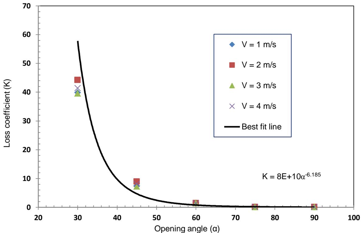
**Fig.15:** Variation of flow coefficient with opening angle at different flow velocities
