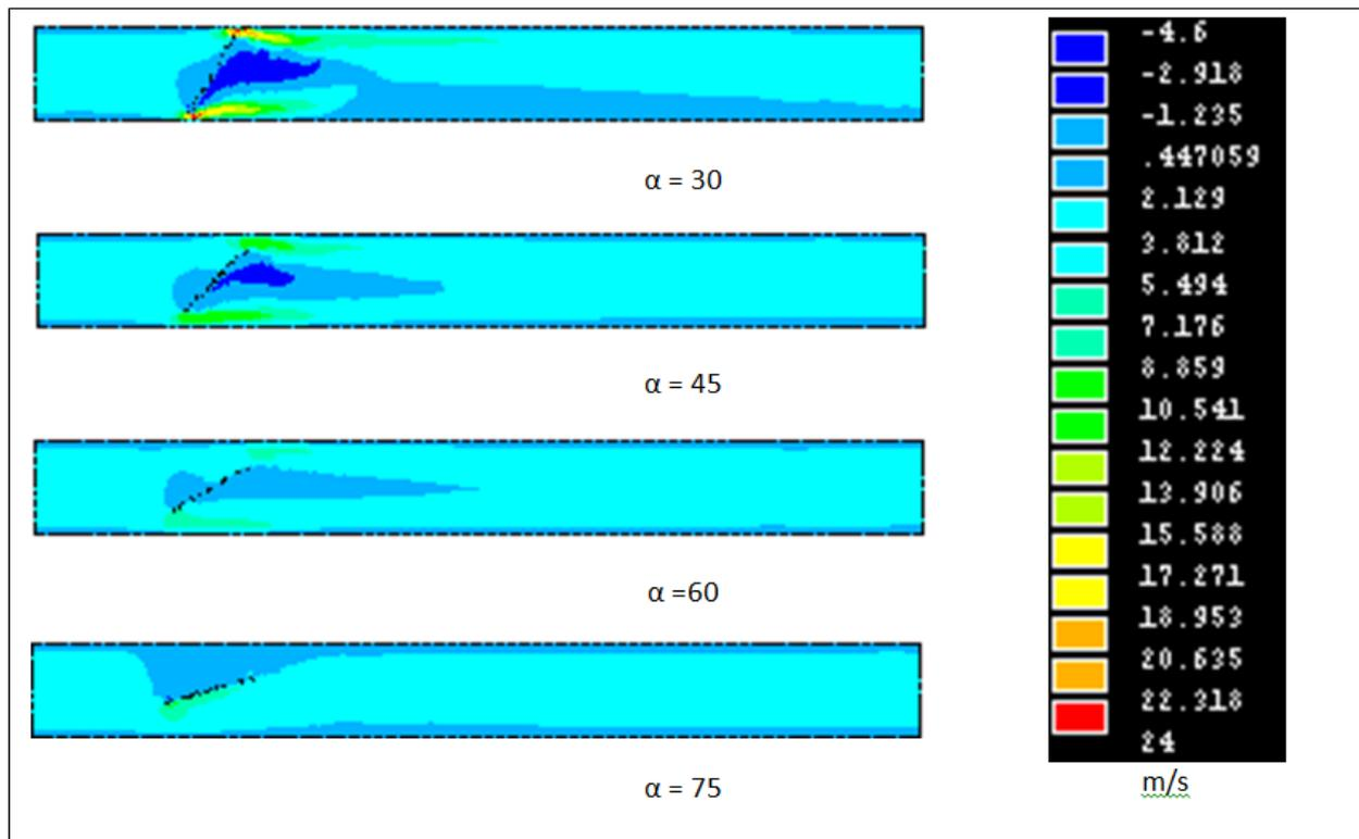
Fig.4: Change of velocity profile with opening angles for 3 m/s inlet velocity
