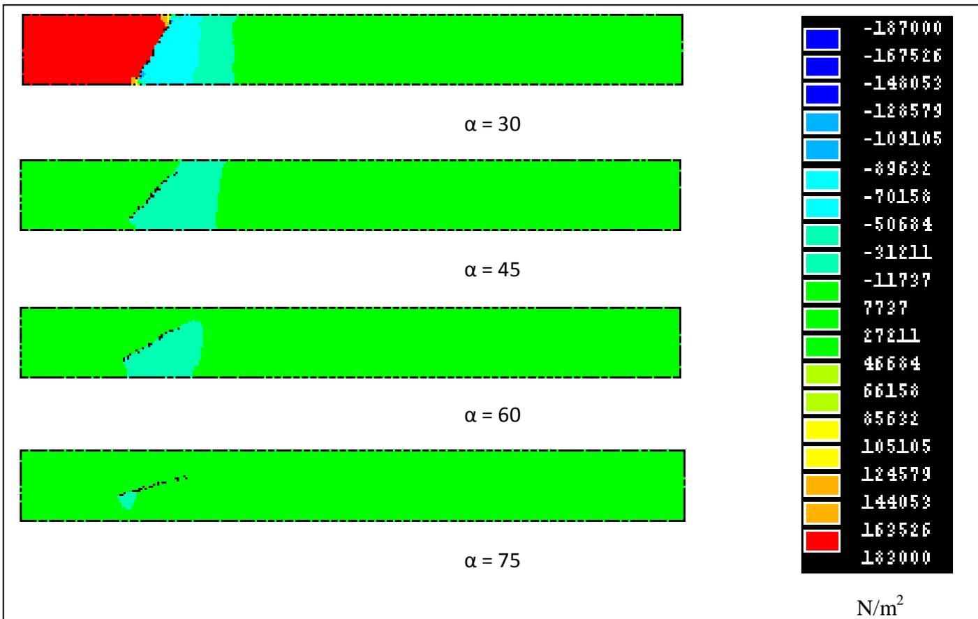
**Fig.8:** Change of pressure distribution with opening angles for 3 m/s inlet velocity
