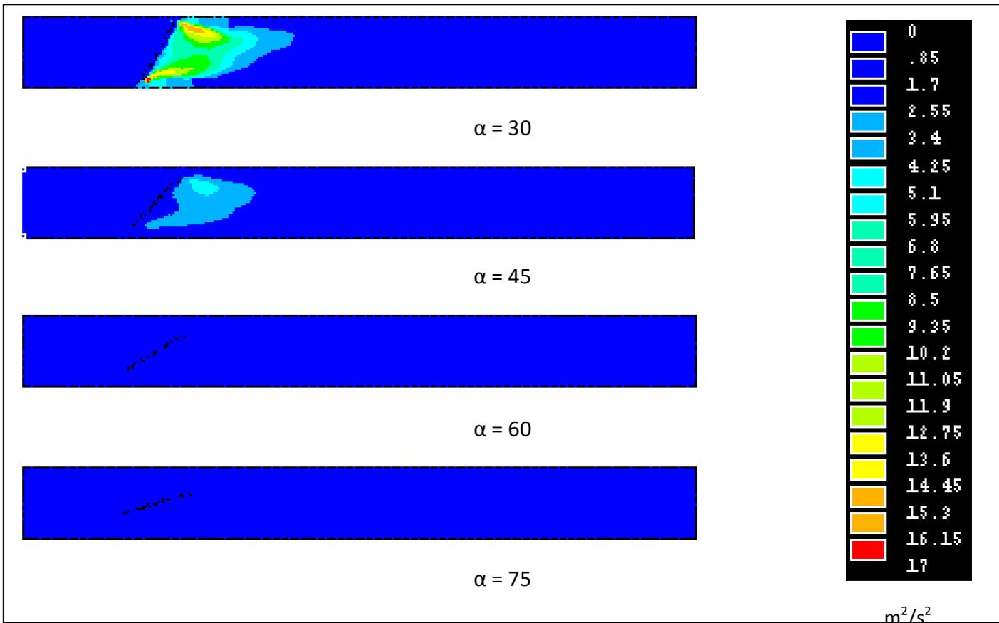
Fig.11: Change of turbulent kinetic energy with opening angles for 2 m/s inlet velocity
