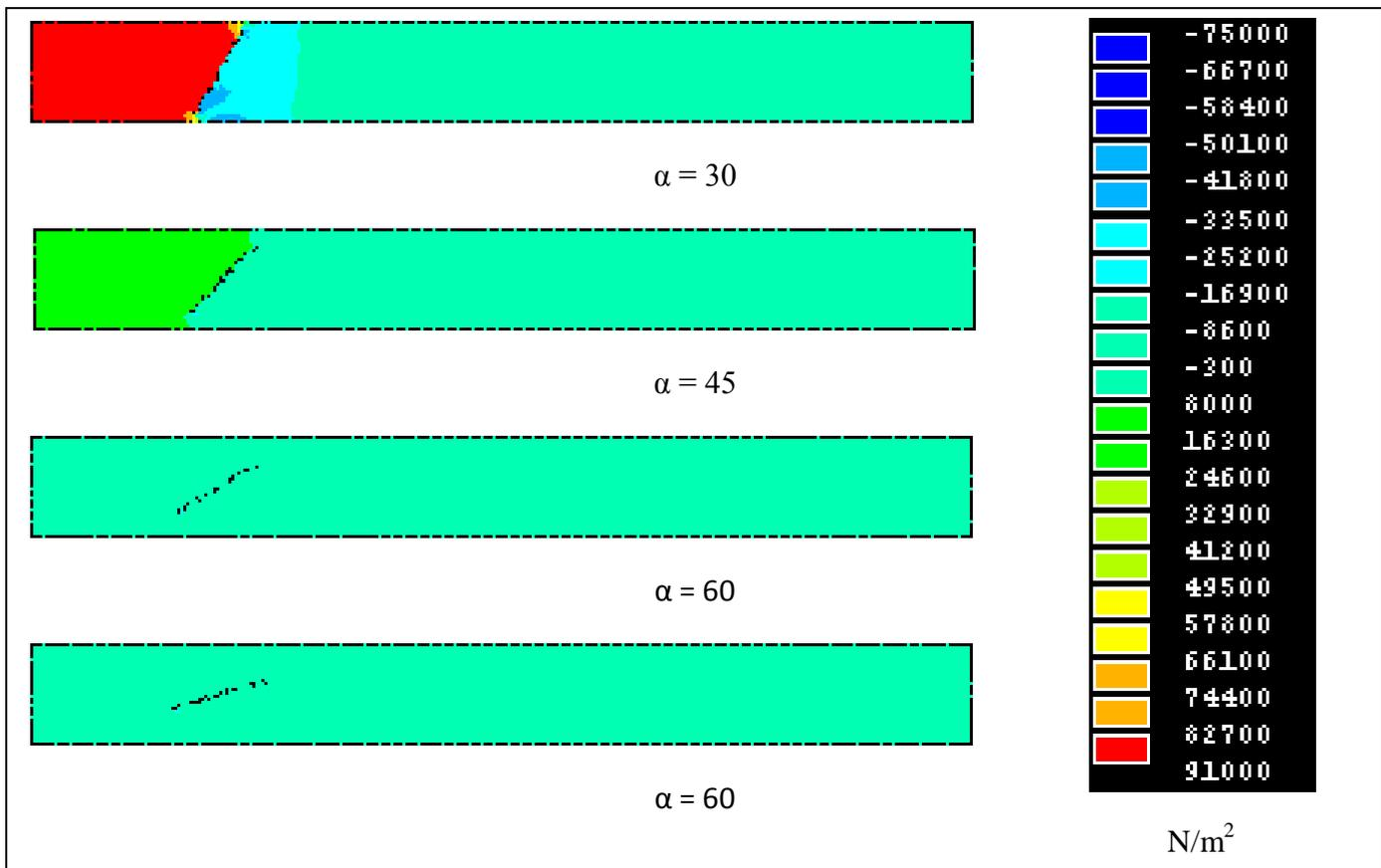
Fig.7: Change of pressure distribution with opening angles for 2 m/s inlet velocity
