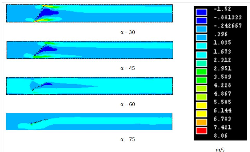
Fig.2: Change of velocity profile with opening angles for 1 m/s inlet velocity
