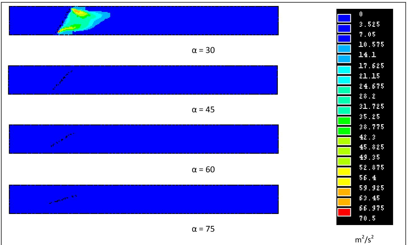
Fig.13: Change of turbulent kinetic energy with opening angles for 4 m/s inlet velocity
