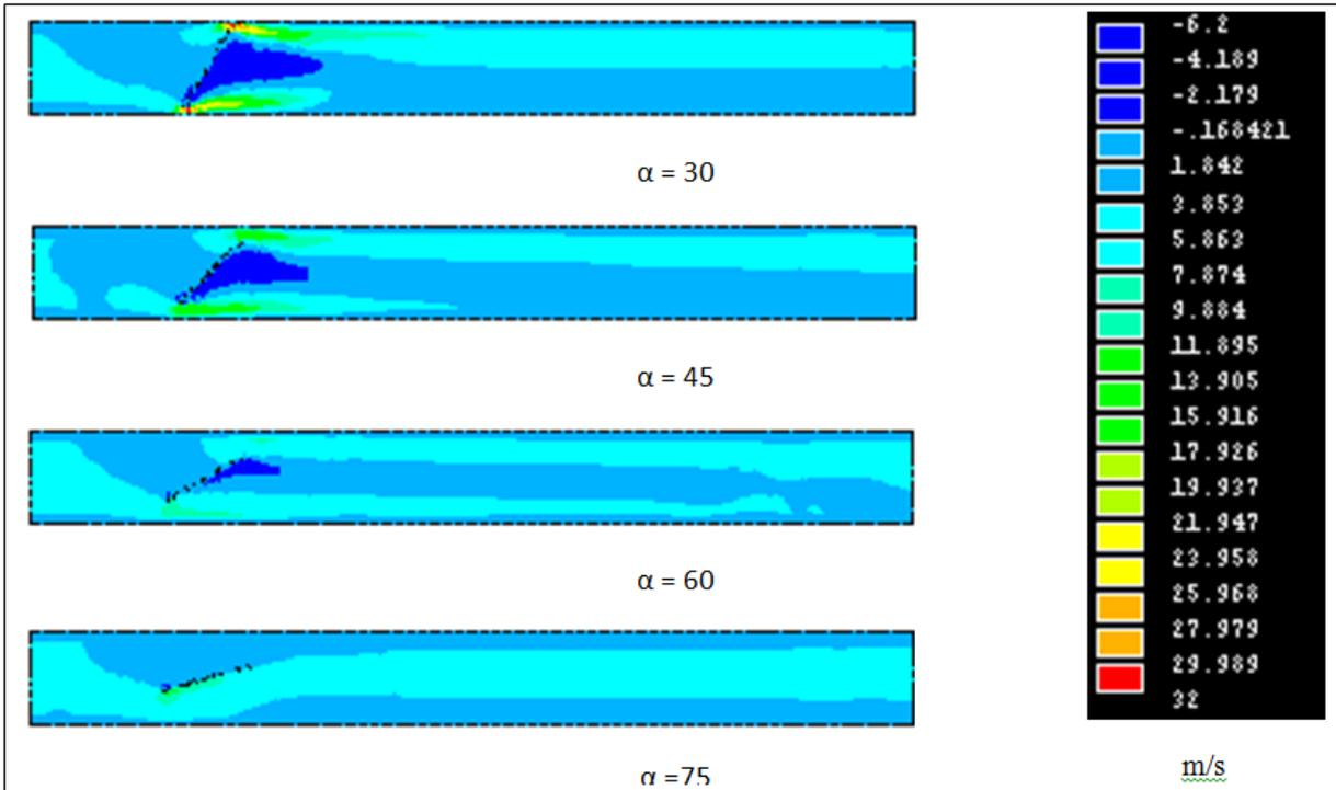
**Fig.5:** Change of velocity profile with opening angles for 4 m/s inlet velocity
