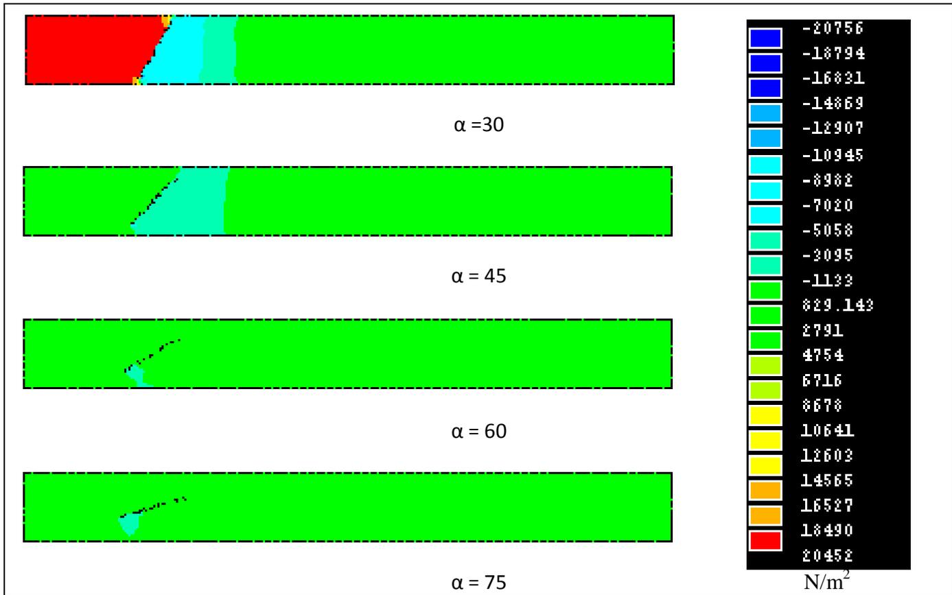
Fig.6: Change of pressure distribution with opening angles for 1 m/s inlet velocity
