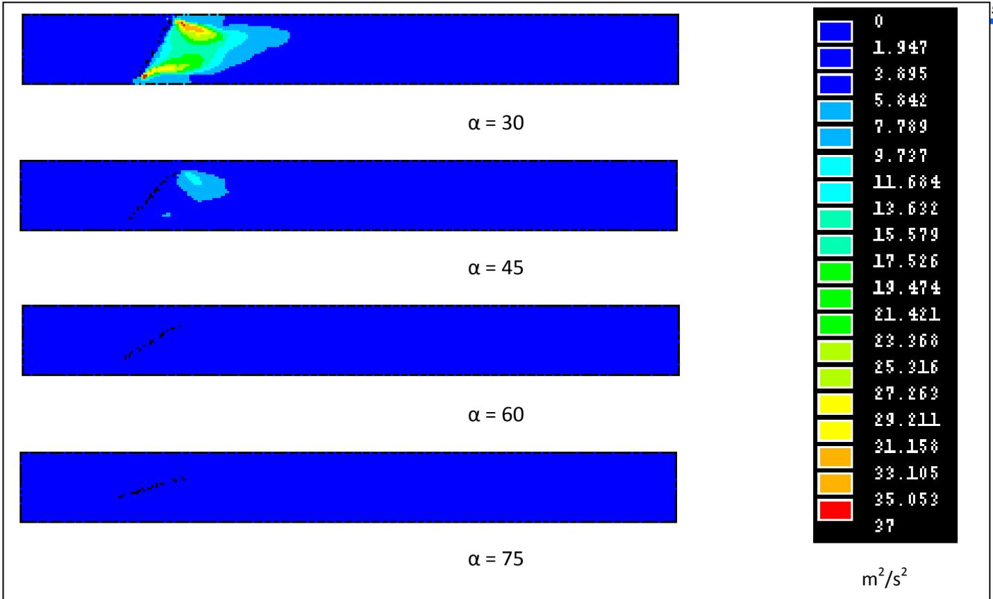
Fig.12: Change of turbulent kinetic energy with opening angles for 3 m/s inlet velocity
