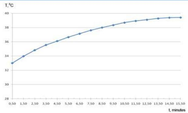
Fig. 4 Kinetics of temperature changes in CCD matrix after switching it on
