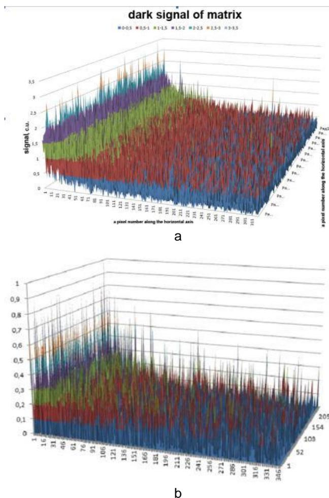
Fig. 1 Topograms of the noise level in CCD-matrixes. (a) Novus-130 BH camera, (b) Mintron OS camera
