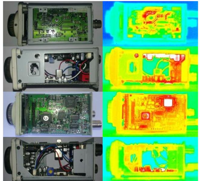
Fig. 5 Appearance (left) and infrared image (right) of electronic components camcorder
