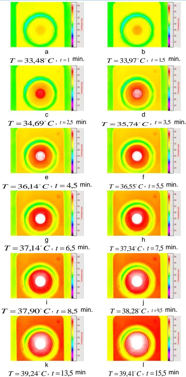
Fig. 3 Thermographic images of the CCD-matrix.
