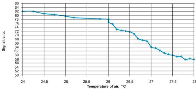
**Fig. 6** Temperature dependence of the useful signal value for the camera Novus-130 BH, when forced ventilation is used.
