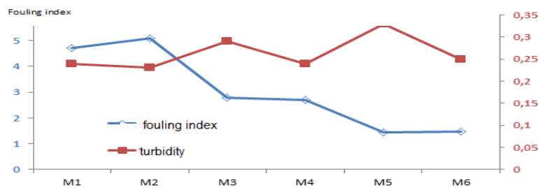
Fig. 6: Evolution of the fouling index based on turbidity
