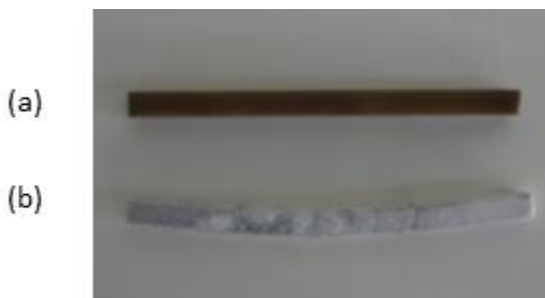
Fig. 10. Photos of (a) as-sintered and (b) crept \alpha/\beta -SiAlON ceramic creep test specimens
