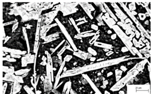
Fig. 14. Back-scattered SEM image of a cross section of the crept specimen (1500 x)
