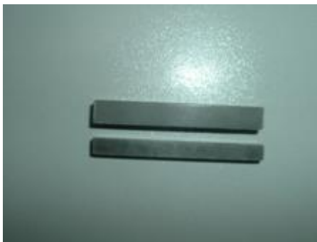
Fig. 6. Photo of as-sintered \alpha/\beta -SiAlON ceramic creep test specimen before and after grinding
