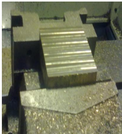
Fig. 5: Pattern of slots after end milling process
