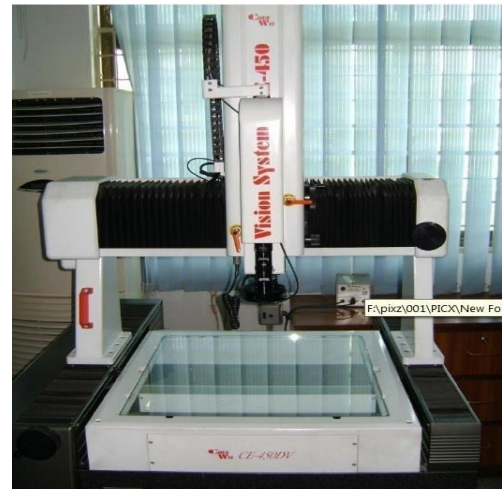
Fig. 7: Coordinate Measuring Machine (CMM) used for the measurement of axial and diameter error
