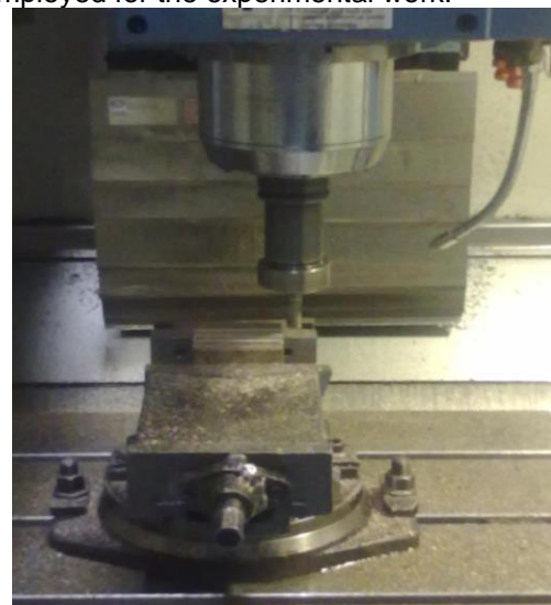
Fig.2: End Milling on the vertical machining center
