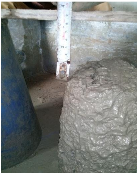
Fig. 5. Workability Measured by Slump Test
