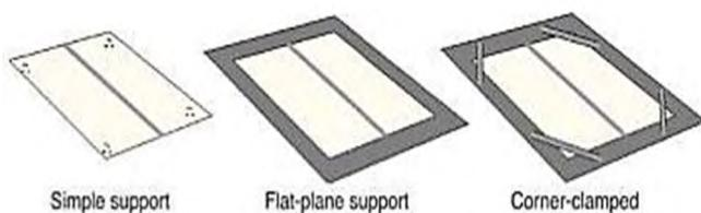
Fig. 2. supporting for butt welding
