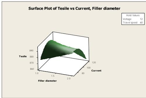
Fig. 10. Contour plot of tensile strength via filler diameter, welding current
