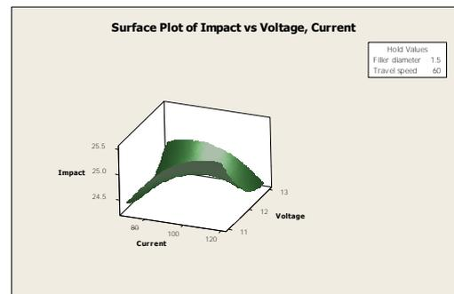
Fig. 15. Contour plot of impact via welding current, welding voltage
