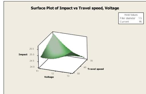
Fig. 13. Contour plot of impact via travel speed, welding voltage
