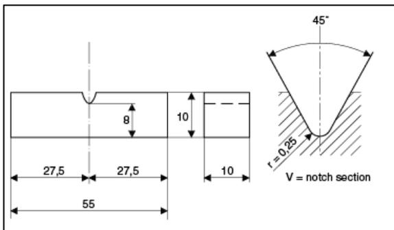
Fig. 11. Charpy V-notch Impact test specimen
