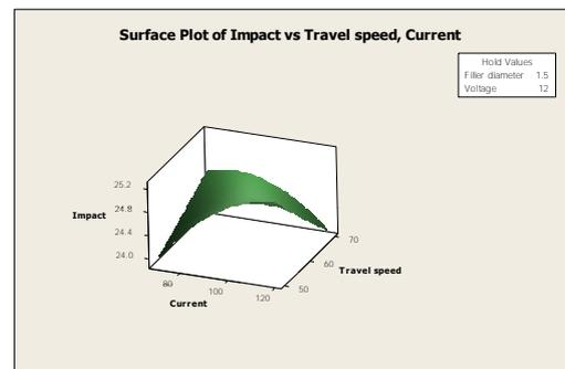
Fig. 14. Contour plot of impact via welding current, travel speed
