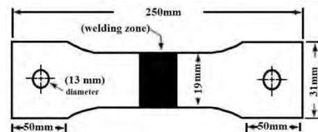
Fig. 3. Tensile sample
