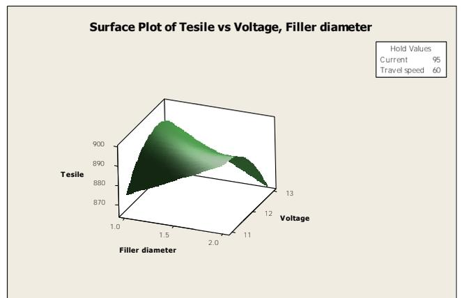
Fig. 9. Contour plot of tensile strength via filler diameter, welding voltage
