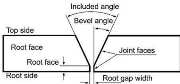
Fig. 1. joint with edges preparation
