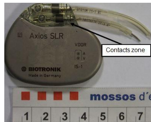
Fig. 2. Contacts zone is the area where the wires enter the housing of the pacemaker
