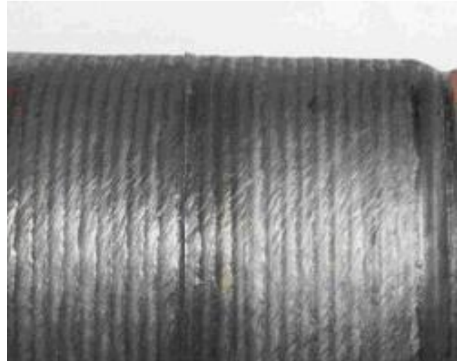
Figure 9. Appearance of the workpiece with 40Ch13 steel layer welded at a current of straight polarity.
