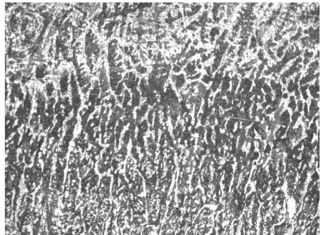
Figure 5. Structure of the welding line. Section #2 (x400).
