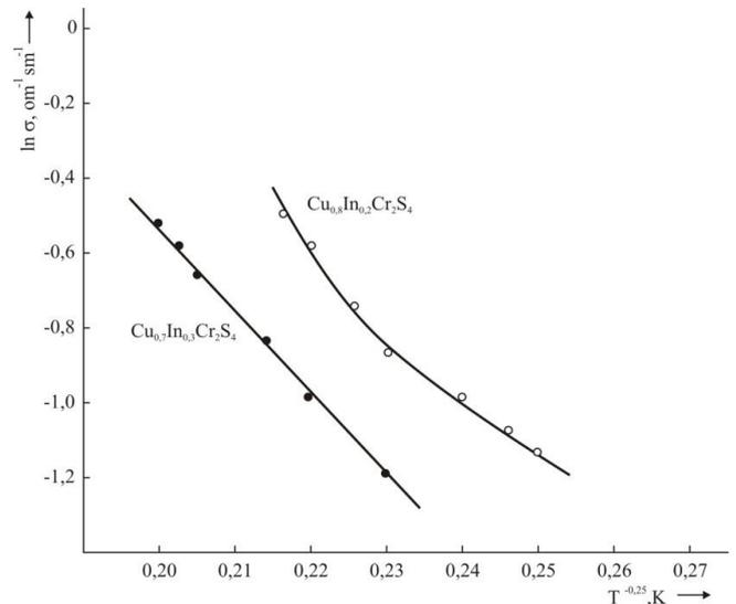
**Fig.4.** The temperature dependence of solid solutions conductivity  $\text{Cu}_{0,8}\text{In}_{0,2}\text{Cr}_2\text{S}_4$  and  $\text{Cu}_{0,7}\text{In}_{0,3}\text{Cr}_2\text{S}_4$  in Mott coordinates ( $237K < T < 623K$ )
