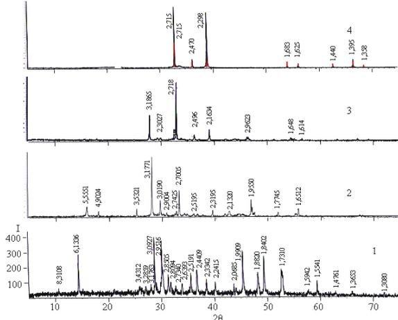
Fig.2. Diffraction patterns of the original components and some alloys of system  $CuCr_2S_4$ -In system
