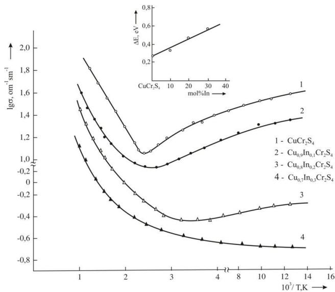
**Fig.3.** The temperature dependence of conductivity  $\text{CuCr}_2\text{S}_4$  and solid solutions  $\text{Cu}_{1-x}\text{In}_x\text{Cr}_2\text{S}_4$  (on the console of dependence of the prohibited zone values on the composition of the solid solutions  $\text{Cu}_{1-x}\text{In}_x\text{Cr}_2\text{S}_4$ )
