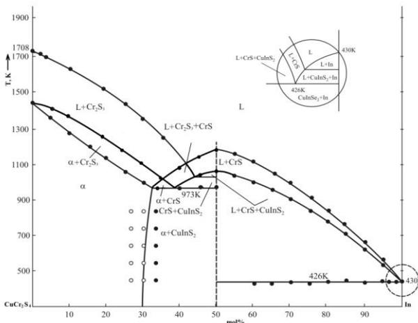
Fig.1. Diagram of  $CuCr_2S_4$ -In system status
