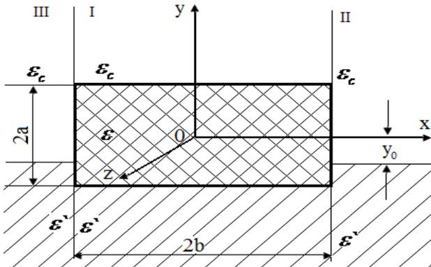
Fig.1. A rectangular waveguide partially embedded in the substrate
