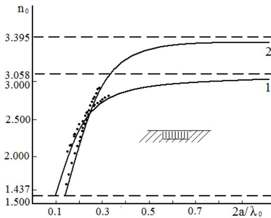
Fig. 3. Basic types of waves of a ruby waveguide embedded in a substrate made of PTFE-4
