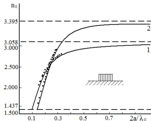
Fig. 2. Theoretical and experimental data for two main types of waves of a ruby waveguide on a substrate made of PTFE-4
