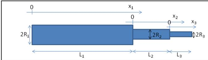
Fig.2. Schematic of the two-step ended rod.
