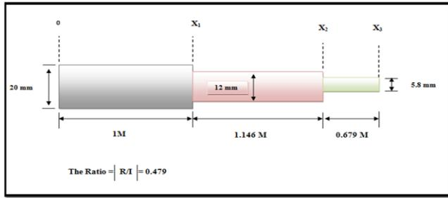
Fig.5. Optimum design with a two-step end bar
