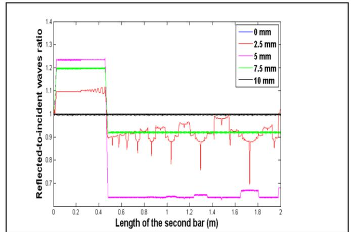
Fig.4. Reduction of the reflected wave in terms of the length of the second bar
