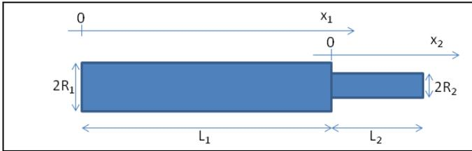
Fig.2. Schematic of the one-step ended rod.
