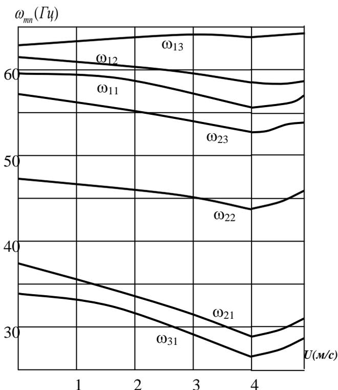
**Figure 4.** Changing the Eigen frequencies of bending vibrations of the speed of the flowing fluid ( $h=0.005$ ).
