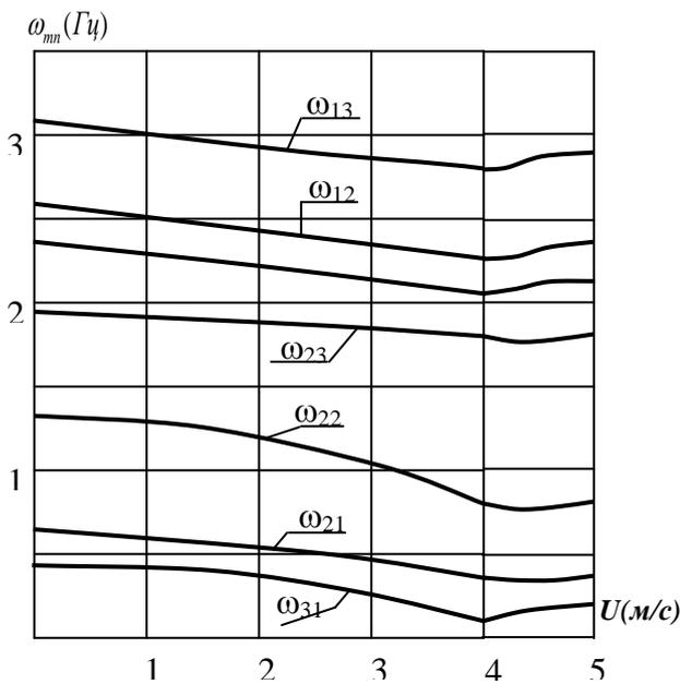
**Figure 3.** Changing the Eigen frequencies of bending vibrations of the speed of the flowing fluid ( $h=0.001$ ).
