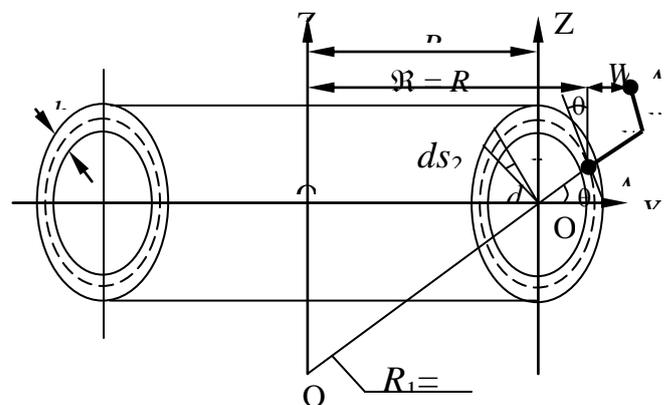
**Fig. 1.** The curved section of the pipeline in the toroidal coordinates
