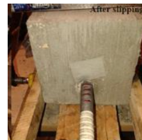
Fig.5. Slipping/pullout of GFRP bars for ECC specimens
