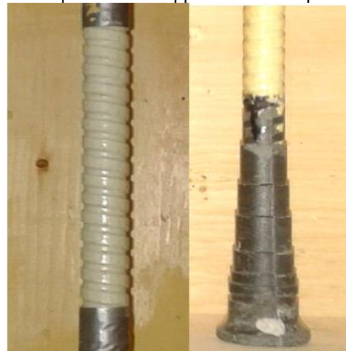
Fig.2. GFRP bars (straight and headed end)
