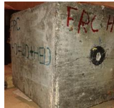
Fig.10. Slipping of GFRP bar for headed end FRC specimens
