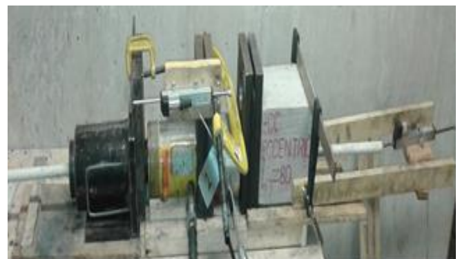
Fig. 4. Pullout test set-up
