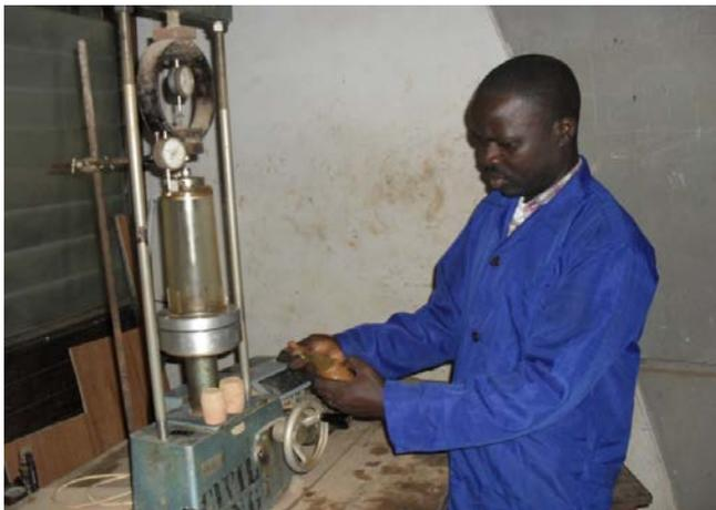
Fig. 1: Triaxial test on soil samples
