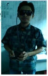
meters, and rapidly vibrating means between 0-1 meters. User (blind) method object testing with the mention approximate distance and match the reference. For indoors with a size of 4 mx 4 m result as the table below.
