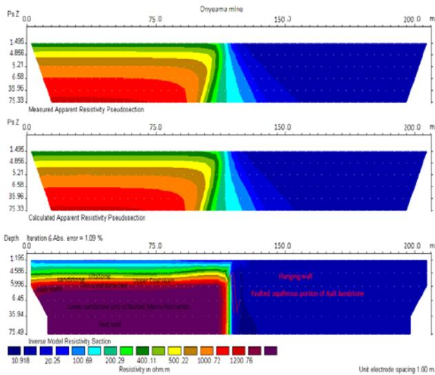
Fig. 6: 2D electrical resistivity tomography imaging along transverse 1, showing faulted Mamu Formation and aquiferous unit of Ajali Sandstone in Onyeama mine
