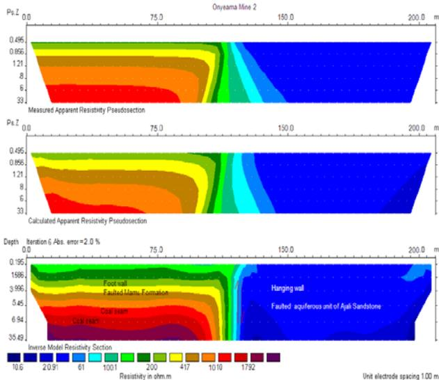
Fig. 7: 2D electrical resistivity tomography imaging along transverse 2, showing faulted Mamu Formation and aquiferous unit of Ajali Sandstone in Onyeama mine
