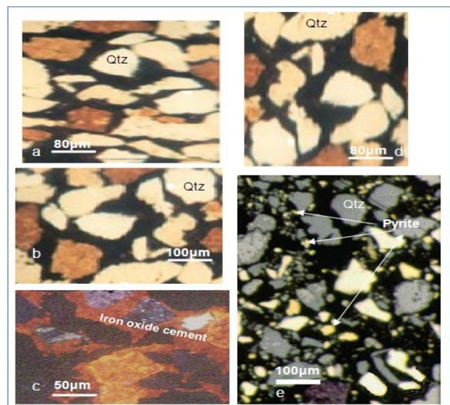
Fig. 5: (a) Fine-medium grained sandstone, (b) Rounded to sub-rounded quartz, (c) Iron oxide cement, (d) Suture-tangential point contact, (e) Disseminated pyrite grain
