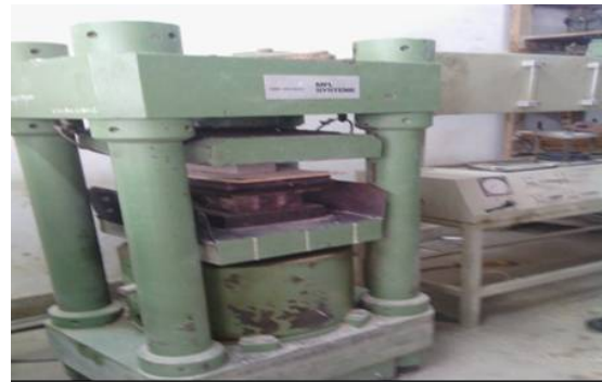
Fig. 2. Compressive test (brick under test)
