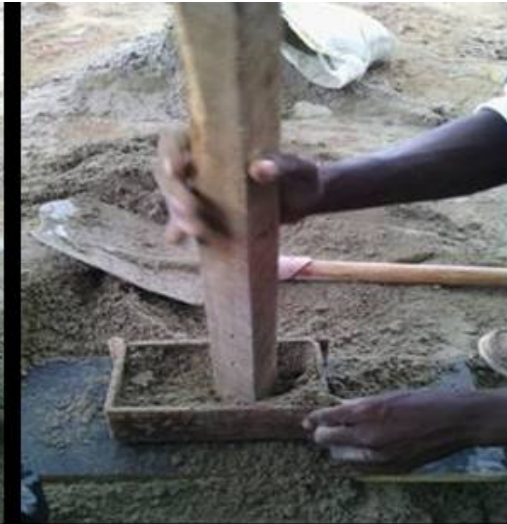
Fig. 3. Compaction by tamping
