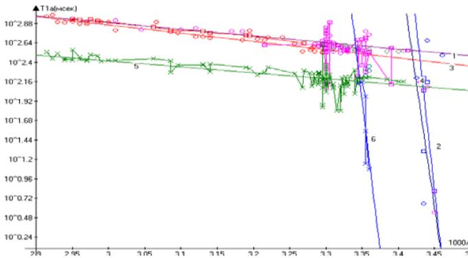
Fig.2. Temperature dependences of relaxation times from inverse temperature  $10^3/T$  in  $\text{CaCl}_2 \cdot 6\text{H}_2\text{O}$  Curves 1,2 –  $T_{1A}$ ; curves 3,4 –  $T_{2A}$ ; 5,6 –  $T_{2B}$
