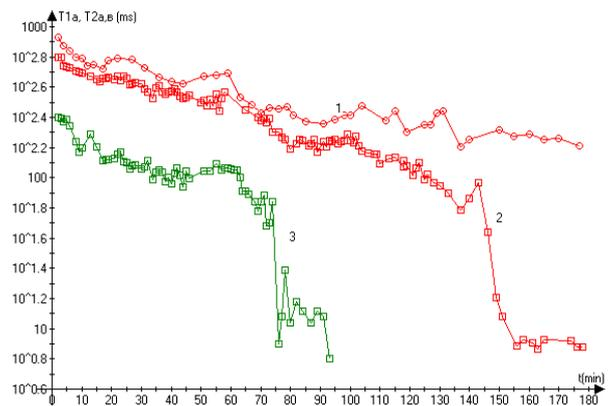
Fig.5. Time dependences of spin-lattice  $T_{1A}$ (curve 1), spin-spin  $T_{2A,B}$  (curves 2, 3) relaxation times from time  $t$  of  $i\text{-C}_{22}\text{H}_{46}$  cooling
