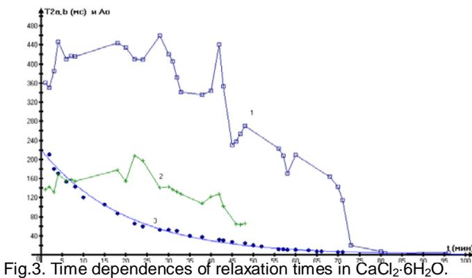
Fig.3. Time dependences of relaxation times in  $\text{CaCl}_2 \cdot 6\text{H}_2\text{O}$ . Curves 1,2 –  $T_{2A}$ ,  $T_{2B}$ ; curve 3 –  $A_0$
