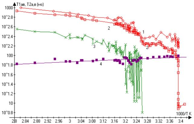
Fig.4. Temperature dependence of spin-lattice  $T_{1A}$ (curve 1), spin-spin  $T_{2A,B}$  (curves 2, 3) relaxation times from  $10^3/T$  K and  $P_{2A}$  proton population (line 4) at cooling of  $i\text{-C}_{22}\text{H}_{46}$ .
