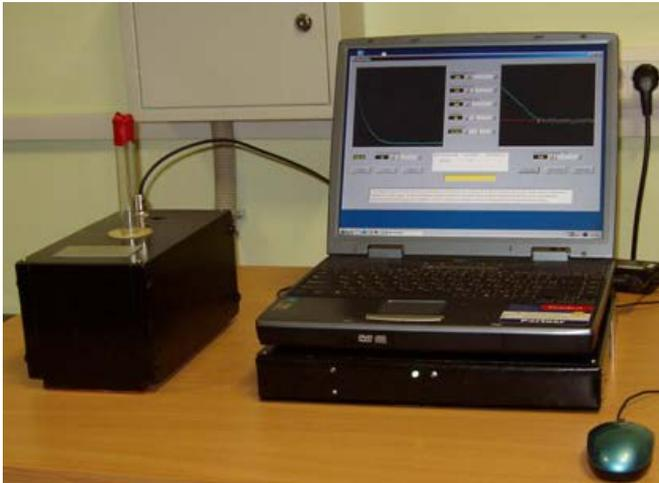
Fig.1. Portable Relaxometer NMR NP-2
