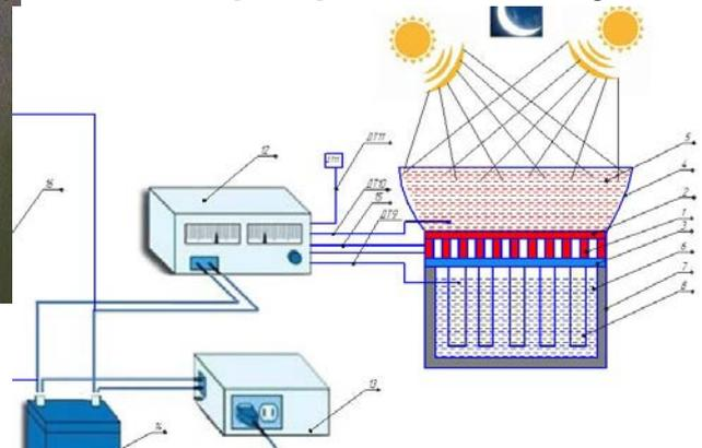
Fig.9 Thermoelectric generator on Seebeck effect and phase transitions
