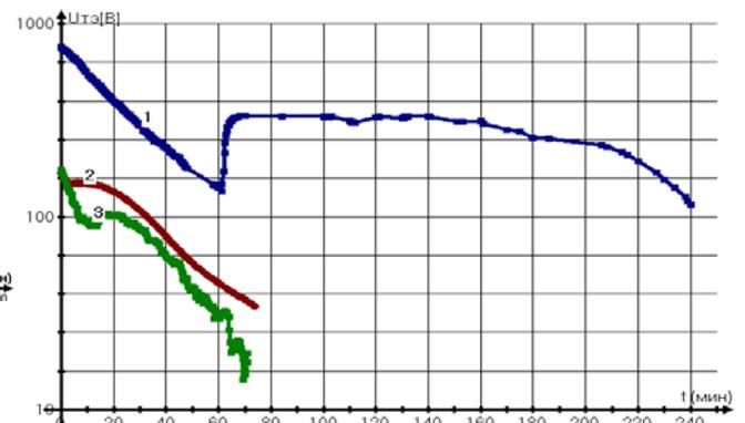
Fig.6. Time dependences of thermoelectricity - electric tension of  $\text{CaCl}_2 \cdot 6\text{H}_2\text{O}$  (curve 1),  $\text{Na}_2\text{S}_2\text{O}_3 \cdot 5\text{H}_2\text{O}$  (curve 2) and  $\text{CH}_3\text{COONa} \cdot 3\text{H}_2\text{O}$  (curve 3) at cooling process
