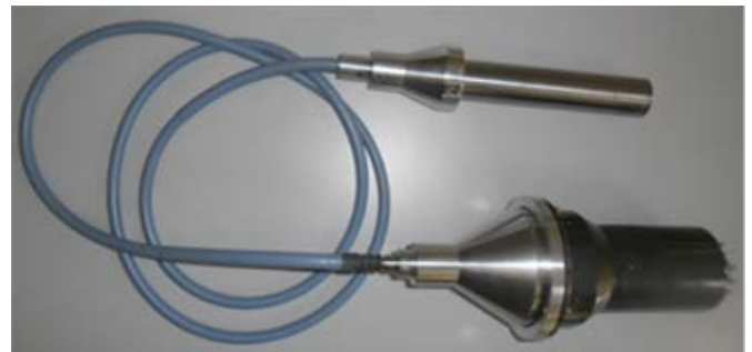
Fig. 1. Proposed remote probe connecting the photomultiplier with the Nal(Tl) detector using an optical fiber.
