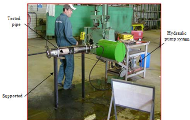
Fig.1. Shows photograph of assembly test rig.
