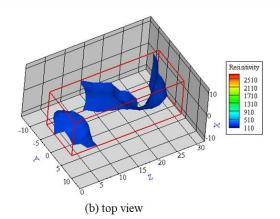
Fig. 7. Distribution of low-resistance abnormal areas in the contour areas of the working face
