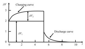
Fig. 1. Schematic diagram of the induced polarization phenomenon in the time domain
