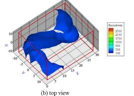
Fig. 6. Distribution of low-resistance anomaly areas on the working face and surrounding areas
